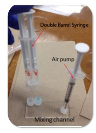
Each device is made of PDMS
